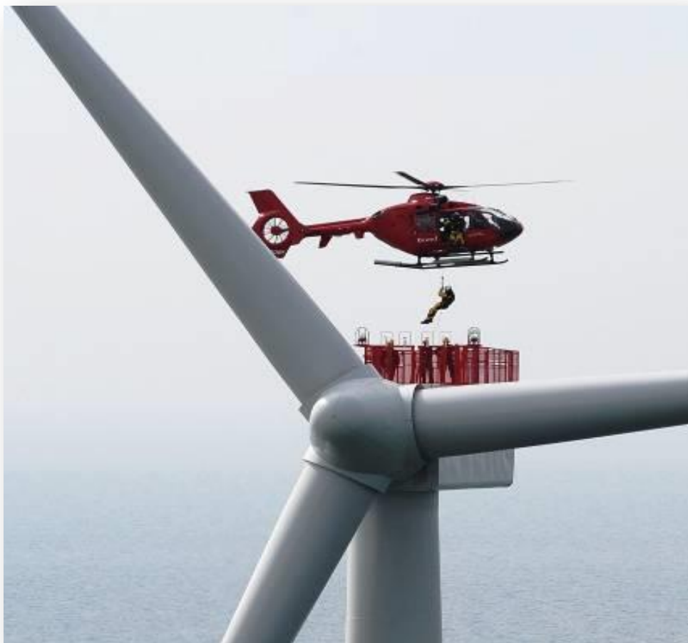
Dropping of a service team @ Greater Gabbard
